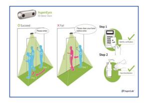
The 3D depth-sensing technology can achieve the high accuracy level to 98% with high tolerance to light and shadow changes, and the overlapping of moving objects.
