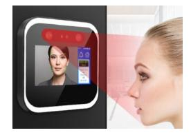
The 5T terminal has the added advantage of a temperature sensors which can check the users forehead temperature before deciding whether to allow entry or not.
