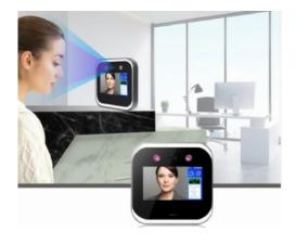
Wiegand input and output for connection to a new or existing access control system for users management.
